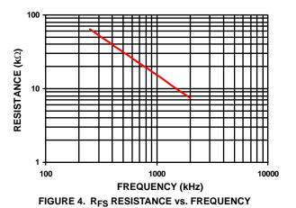
$Fs[Hz] \approx 1.178 \times 10^{10} \bullet R_{T}[\Omega]^{-0.973}$  (R<sub>T</sub> TO GND)
