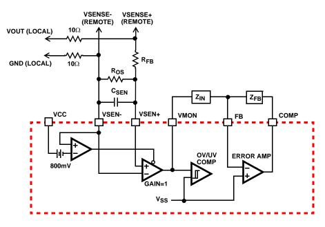
FIGURE 6. SIMPLIFIED UNITY GAIN DIFFERENITAL SENSING IMPLEMENTATION
