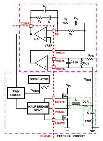
FIGURE 10. VOLTAGE-MODE BUCK CONVERTER COMPENSATION DESIGN
