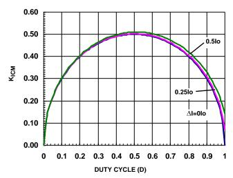
FIGURE 12. INPUT-CAPACITOR CURRENT MULTIPLIER FOR SINGLE-PHASE BUCK CONVERTER
